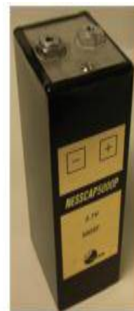
Fig 2.3: Nesscap capacitor module rated at 5000 Farads
